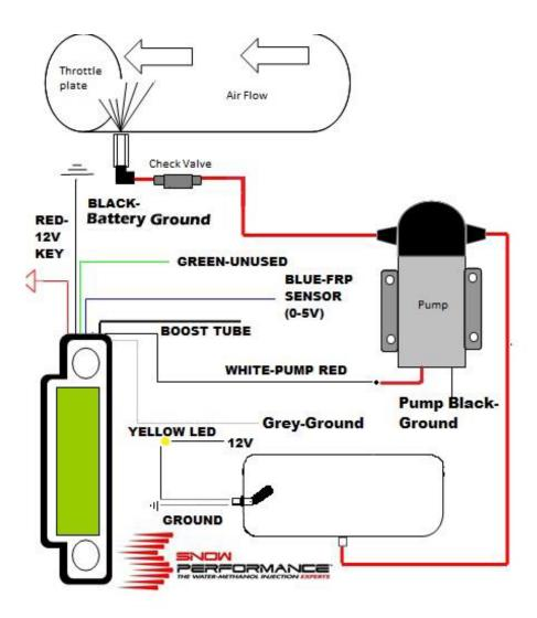
**Step 1 Stage 3 Controller Wiring/Boost Source**
