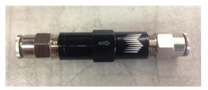
Braided line kits - Fit the NPT thread to 4AN adapters in each side of the check valve using E-6000 sealant on the NPT threads only. Connect the 5 foot section of braided line from the pump outlet to check valve inlet and the 1' or 2' section of braided line from the check valve outlet to the nozzle holder inlet.
