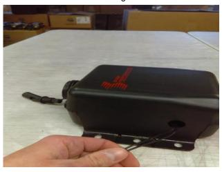
Step 3: Remove the cap from the tank and feed/pull wires through hole until level sensor is seated against plastic stopper.
