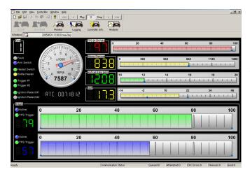
This screen graphically displays the operational status of the MAXIMIZER-II in real-time. To access this screen, simply click the Monitor button on the Main Screen or type M.
