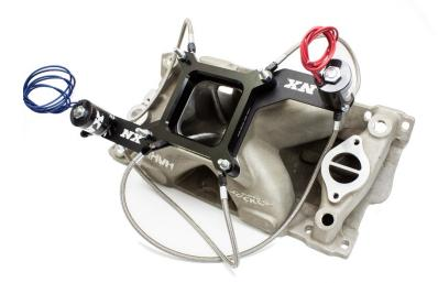
NOTE: As you can see in the (Illustration B), the fuel and nitrous ports on the plate are on opposite corners of each other. Please advise when installing the lines on the plate and make sure they are installed on the right ports for you solenoids.
