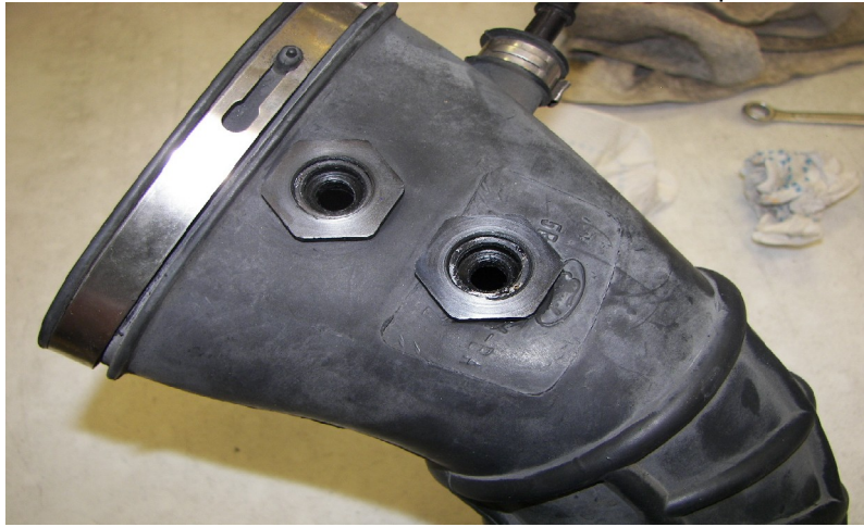
Twin nozzle setup in the stock intake tube of 2007 Mustang using 2 nozzle mount adaptors. This locates the nozzles immediately before the throttle body.
