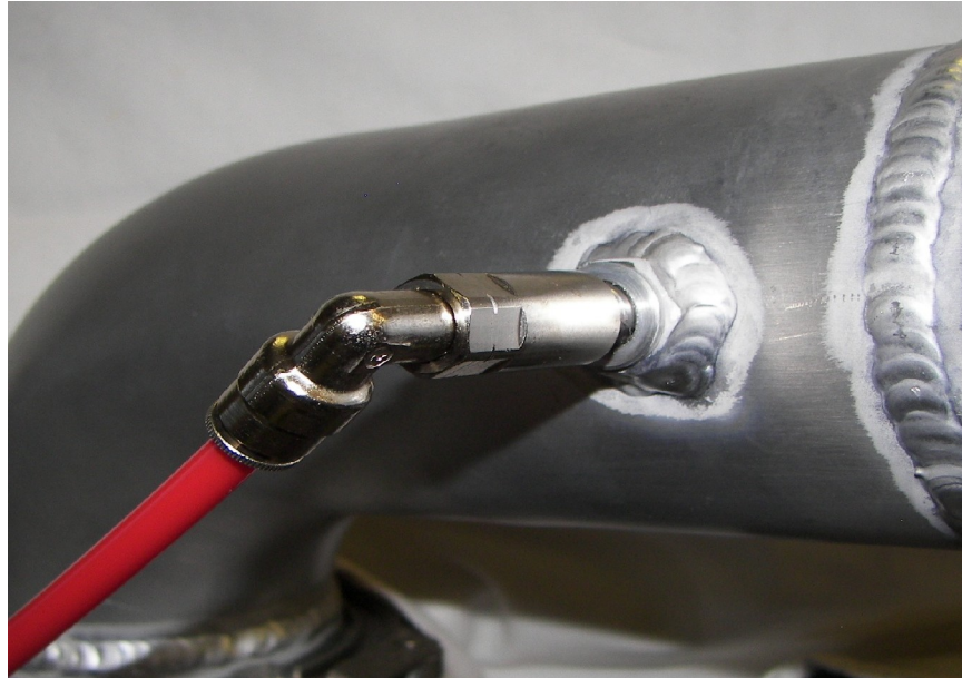
Aluminum weld-in bung shown.
