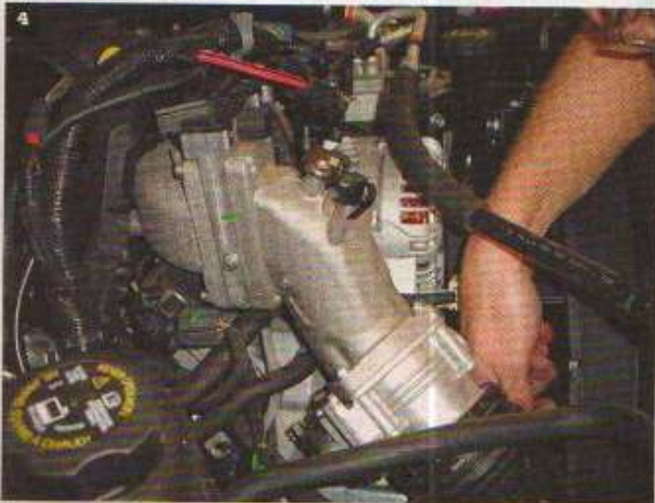
To prepare for the installation of the MPG-MAX, it was necessary to remove the aluminum inlet elbow.
