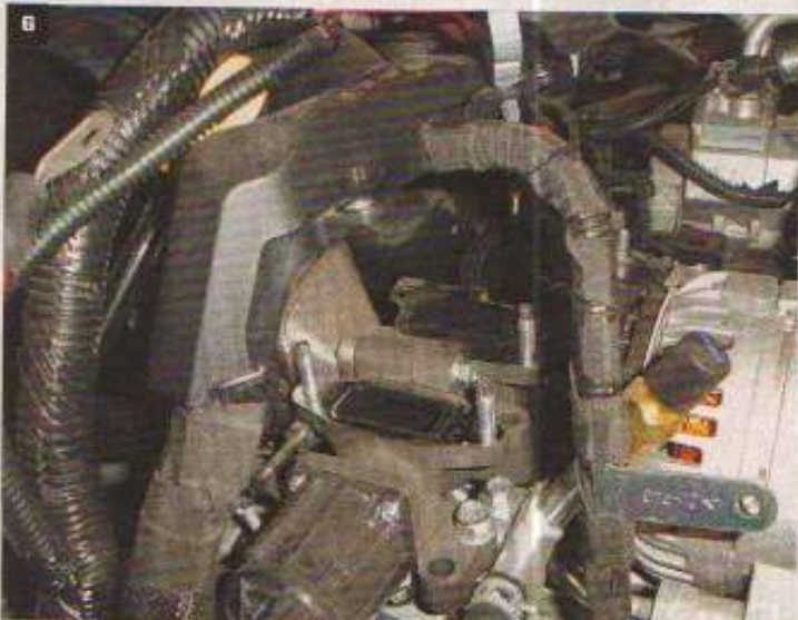
Here is a shot of the removed intake manifold. Take care to cover the inlets to protect them from debris. Note the soot buildup from the EGR system.
