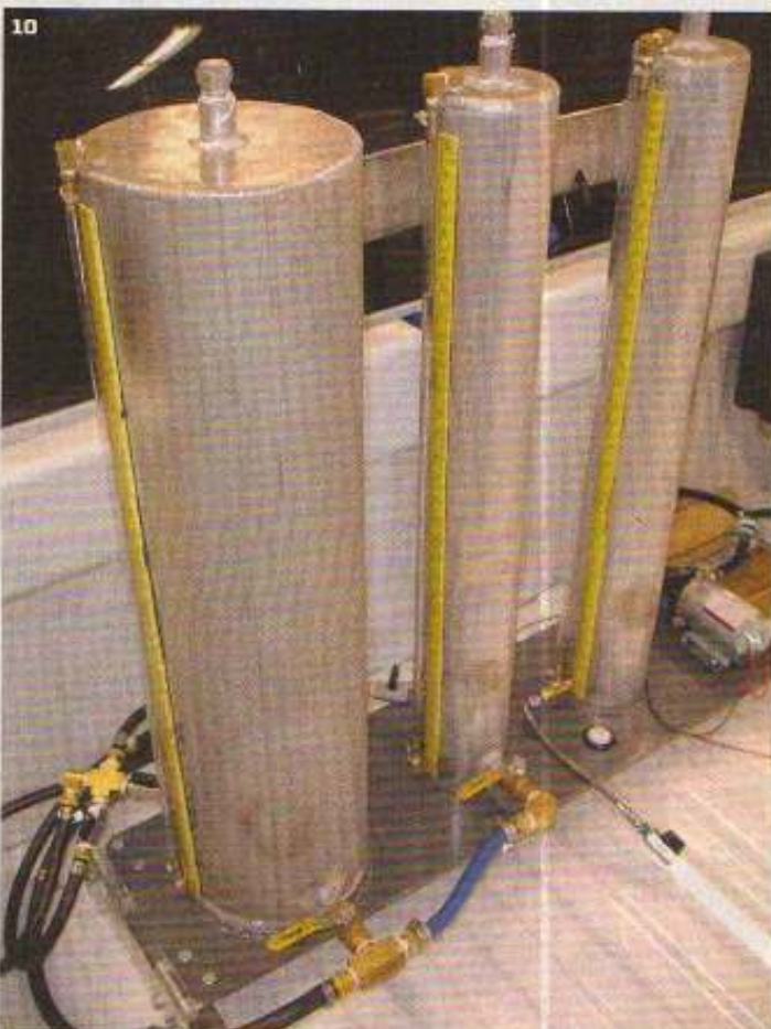
To properly measure the amount of fuel and water-ethanol supplied to the motor during testing, ICM designed these fuel tanks and mounted them in the bed of the truck. The dedicated fuel tanks allowed precise measurements of the fuel usage.
