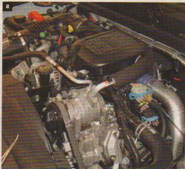
Impressive even in stock trim, the 6.8L Duramax motor produced 245 hp and 556 lb/ft of torque at the wheels.
