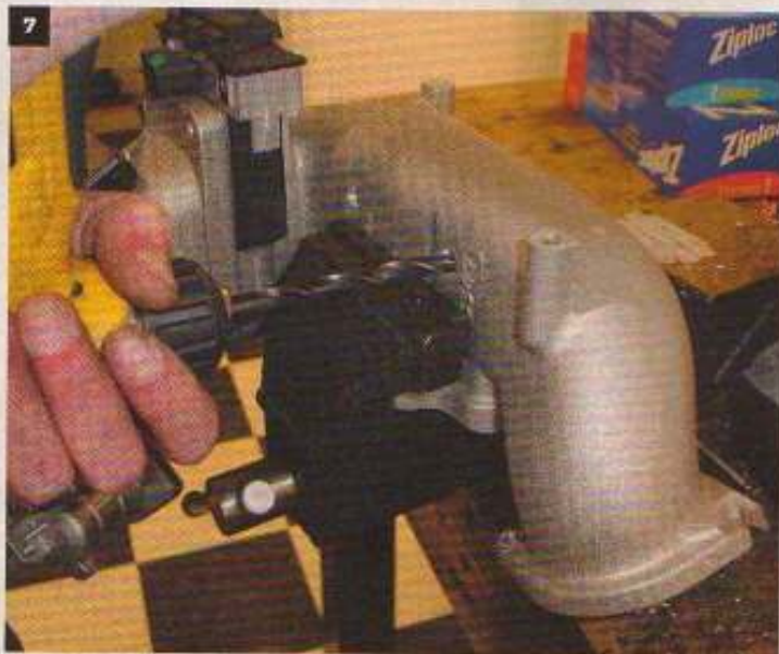
Once removed, the intake elbow was drilled and tapped to accept the supplied nozzles.
