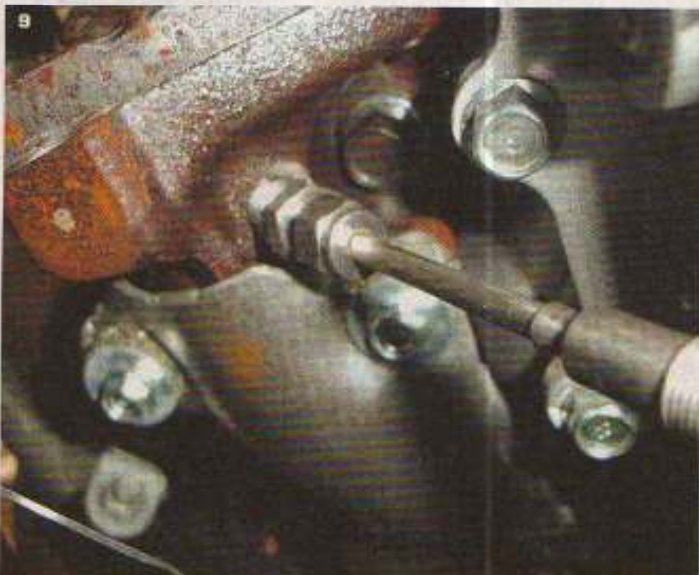
Exhaust gas temperatures are critical on modified diesel applications, especially ones that tow, so ICM installed this EGT probe to log the temperatures during testing. A full set of gauges is always recommended on serious tow or modified diesels.
