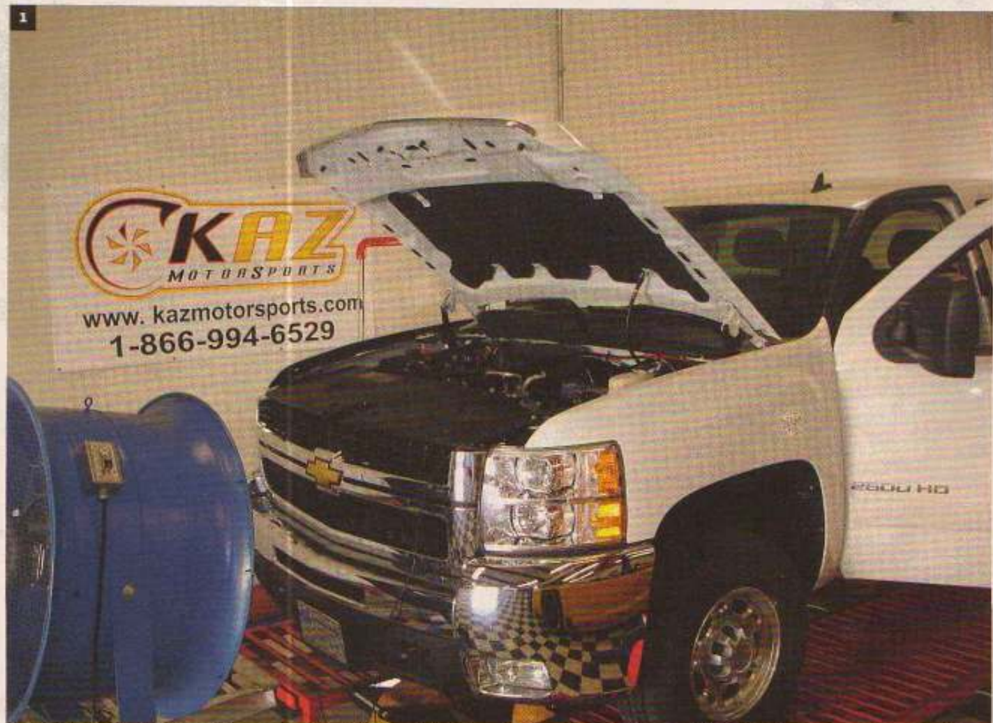
To illustrate the performance and economy offered by the MPG-MAX system from Snow Performance, this 2008 Silverado was first run on the chassis dyno.
