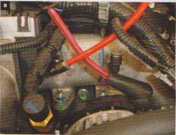
Here, the nozzles have been inserted into the elbow. Two nozzles allow the motor to run in "MPG" or "Power" mode. The two can also be combined to offer additional power.
