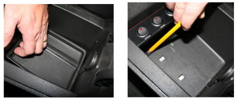
Using a 3/16" drill bit, drill small holes for the mounting clips to hold the switch panel in place, then place the switch panel in place using the mounting tape and the small clips to hold the panel in place and re install the rubber liner in the bottom of the console.
