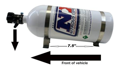
Mounting the bottle in this manner will allow the internal siphon tube to be covered with liquid nitrous at all times and properly supports the bottle. Refer to the chart below to determine the suggested bracket spacing.
