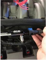
4. Next, remove the 2x 10mm nuts on top of the intake that hold the large hose in the picture, in place. Mount the solenoid bracket on the 10mm stud closest to the front of the car. (See pic.) Attach the solenoids to the bracket using a standard Phillips head screwdriver.
