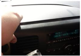
4. Once the dash is removed you will need to drill a small hole (3/8" recommended) for the wires to pass through, you can see the two small holes where the mounting tabs go and recommended area to drill hole.
