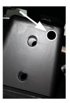
5. Place switch panel in the small compartment and push tabs through the bottom to secure switch panel to the dash bezel.
